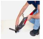
2. Wrap chain around pipe and engage nearest pin in upper jaw hooks.
